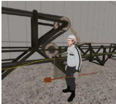
Caught-in accidents (high-speed conveyor belt)
