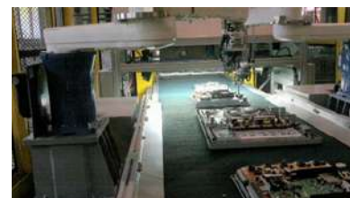
Robot unscrews flat-screen TVs
