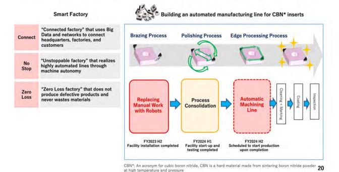
Next please. This represents an example of a smart factory in the Metalworking Solutions business. As part of the DX initiative, progress is shown here using the example of an automated line for a product called CBN insert.
