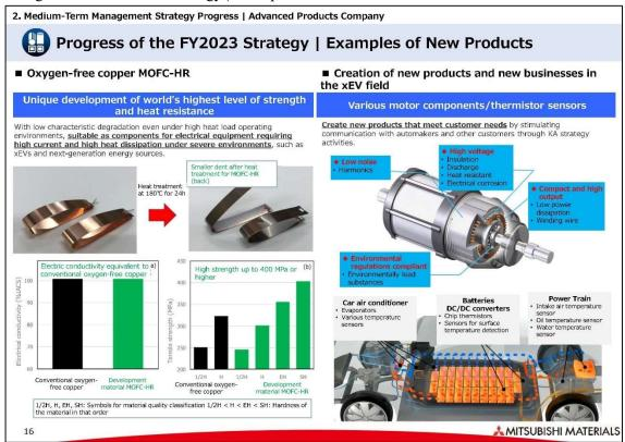
Page 16 shows examples of typical products of Advanced Products Company. The left side of the slide is about oxygen-free copper MOFC-HR. I am omitting the details since we have already issued a press release, but this material has the same electric conductivity as conventional materials, but with higher strength.
