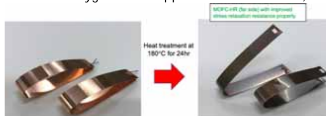
Newly developed MOFC-HR, ideal for high current busbar and terminals, etc., for xEVs appliances
