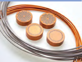
Superconducting wires often used in medical devices for applications such as MRI and international science projects
